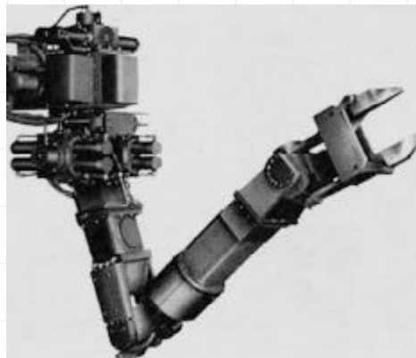
Fig. 1.13 The Arm, a 6 DOF bilateral force-feedback manipulator
