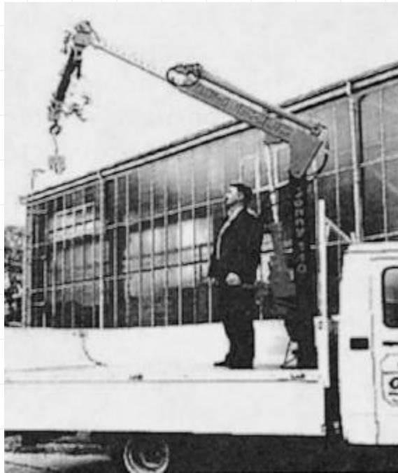
Fig. 1.1 (a) A Kuhnezug truck-mounted crane Reprinted with permission from Kuhnezug Fordertechnik GmbH.
